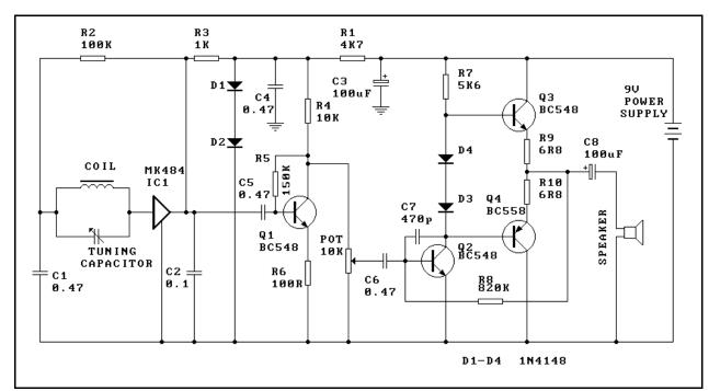
**If It Does Not Work.** Check that the diodes are all in the correctway. Are the resistors in the right places. Check that
